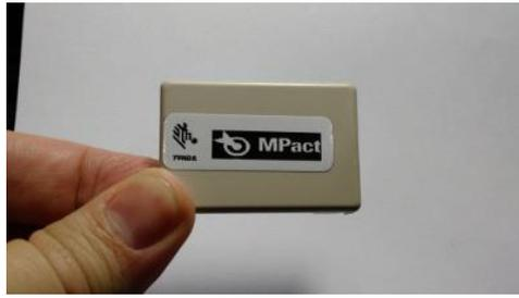
**Figura 1:** Sensor *MPact Beacon BLE*
